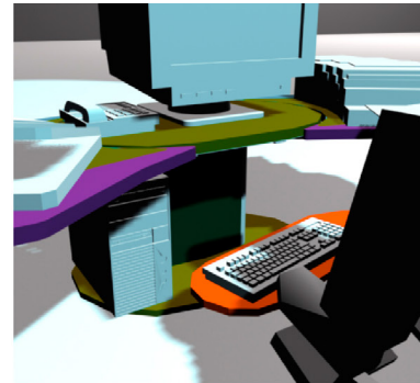
Figure 32. Images of the desk proposal with hinged arms and lowered keyboard support (Authors: C. Cavaleiro, J. Moreira and P. Carvalho).
