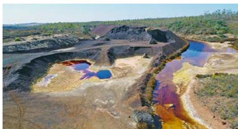
The project focuses on one of the world's most serious environmental problems, known as acid mine drainage, which is a process associated with the exploitation of metals. The general idea is the characterization of the natural nanoparticles that result from this process, since they contribute to mobilization of toxic elements.
